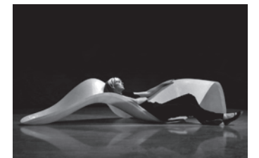
Achim Menges' Lounge Landscape furniture piece, constructed from novel composite material systems consisting of a 3D spacer textile sandwiched in a stressed glass fibre skin. (HfG Offenbach)
