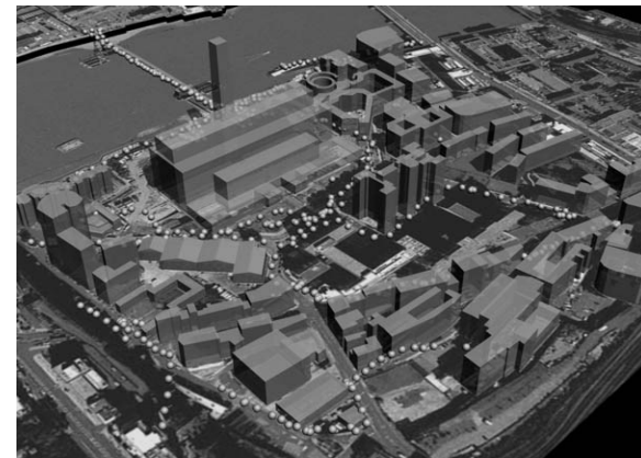
Figure 2: Positions of measurements of air temperature, relative humidity and wind velocity as recorded by GPS around the Tate Modern site in south London.
